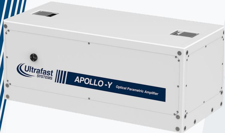
The **APOLLO-Y** Optical Parametric Amplifier is designed to extend the tuning range of an ultrafast Ytterbium amplifier from the UV to the NIR. It is optimized to work with Ultrafast Systems' spectrometers – [HELIOS](#), [EOS](#), [HALCYONE](#), etc. High stability and high efficiency are achieved through three step amplification of a white-light supercontinuum, and all nonlinear crystal tuning, optical delay compensation, and wavelength separation is fully computer controlled.
