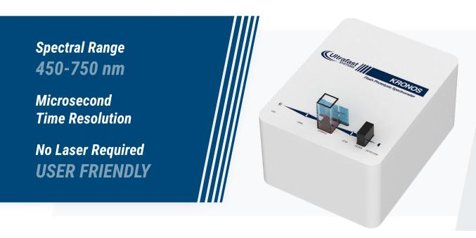
**KRONOS** is a portable flash photolysis spectrometer designed for transient absorption and emission measurements on the microsecond and longer time scales. It is intended as a chemical kinetics experiment in university or high school teaching laboratories. KRONOS can measure solid and liquid samples in absorption as well as emission modes. KRONOS utilizes a Xe arc flash lamp with bandpass filters as an excitation source.
